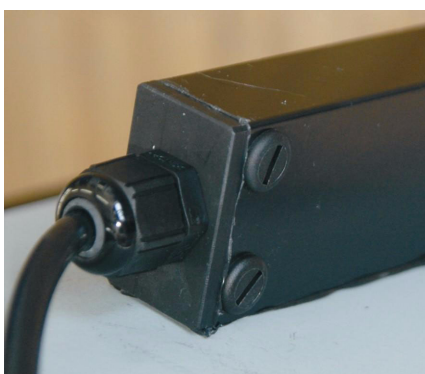
Fig. 4: Cover cap of the cable gland
