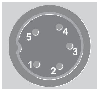
Fig. 7: Assignment of the plug for function signal and external release (contacts at rest)
