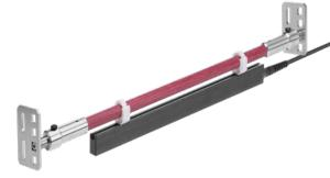
The bracket with perforated plates allows the bar to be latched into the various positions of the perforated plate. The possible positions are determined by the various available designs of the perforated plates. The perforated plates are attached to the stable parts of the machine. This will absorb the force of the spring-loaded spigot and the bar is moved into a stable position.
