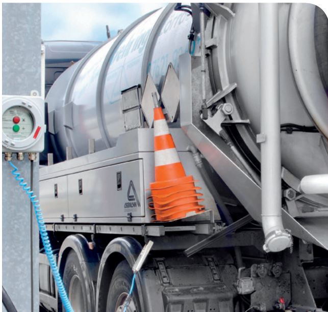
Active grounding for tanker trucks
