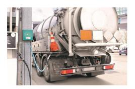
Photo: Truck grounding with TERRABOX
